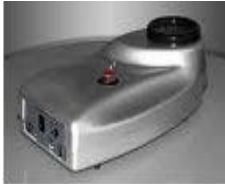
Figure C-1: Photograph of GDV Camera pro version 3 designed for measuring drops of liquid. There is a special syringe holder that is placed on top of the black ring which can hold a drop from a syringe just above the glass plate where the measurement is performed.
